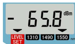
レベル設定後の表示 Measurement value after buzzer reference level is set.
